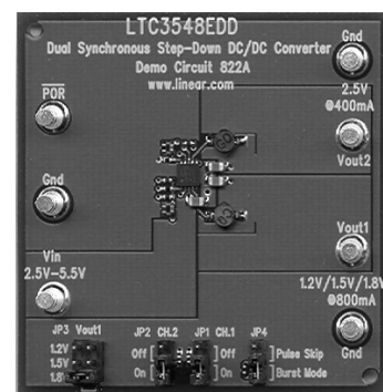
Figure 11. Less than 150mm 2 is needed for two DC/DC converters (LTC3548).
