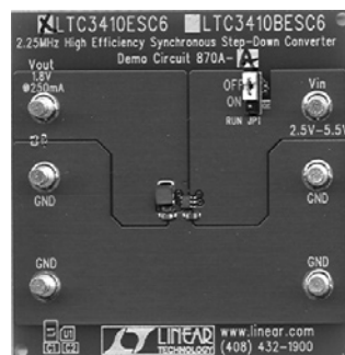
Figure 3. The LTC3410 supplies 300mA without taking much space.
